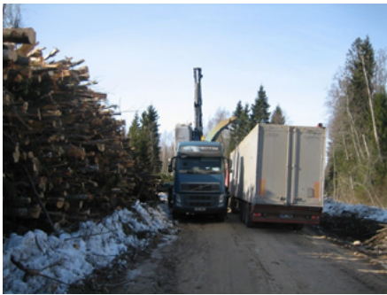
Figure 5.9. Chipping of logging residues into a truck bed, (photo P. Muiste)
