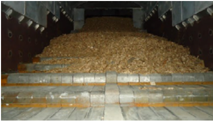
Figure 7.2. Moving grate for burning wood fuel [40, 41]
